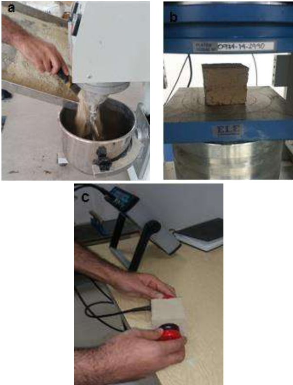
Fig. 3. a) Mixing process, b) Compressive strength test, c) UPV test
