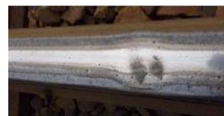
Figure 5. An example of scour defect that can happen in the rail [16].
