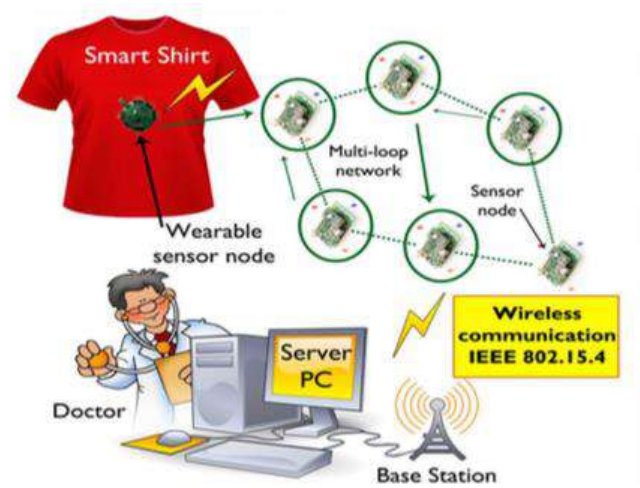
Figure 7 A wearable smart shirt system architecture
