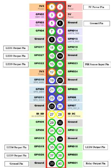
Figure 11. GPIO pins layout for proposed system
