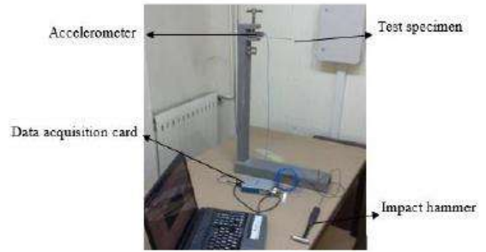
Fig. 2. Experimental set-up for vibration tests
