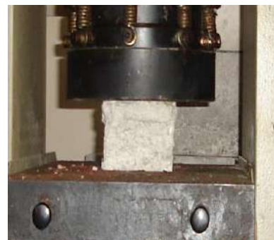
Fig.3 - PAPERCRETE CUBE IN PLACE FOR COMPRESSION TEST
