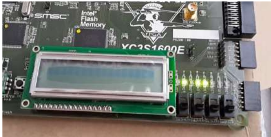
Figure 6. Display of 88 in binary at LED output of the FPGA
