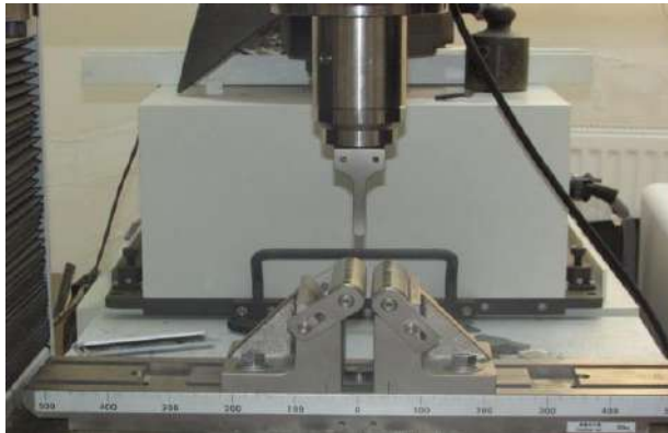
Fig. 3. Test setup for the three point bending test
