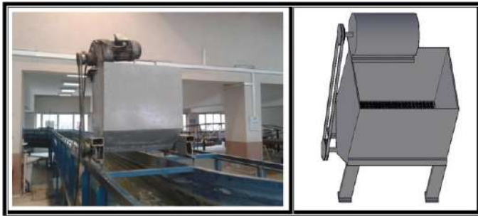
Fig. 10. Portative machine that provide solid material supply to the channel
