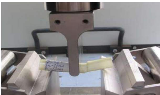
Fig. 4. Different lengths of specimens of glass/epoxy subjected to the three point bending test: a) L=250mm, b) L=80mm
