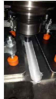
Fig. 2. A sample for FS welding
