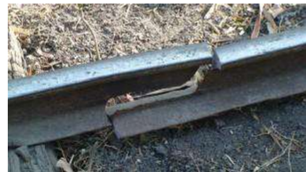
Figure 2. An example of the rail fracture [17].
