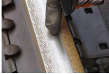
Figure 6. An example of wear defect that can happen in the rail [18].
