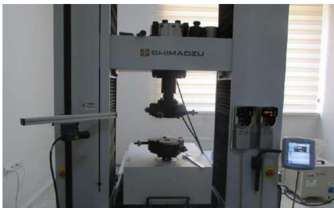
Fig. 7. Test setup for the torsion test
