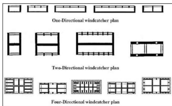
Fig. 5. The plans of different sorts of wind-catchers [9].
