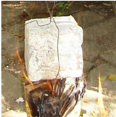
Fig.5 – Cube Sample Held in Flame
