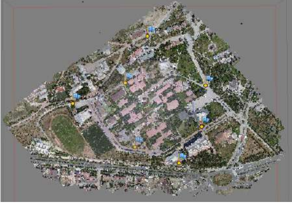
Fig 5. 3D point cloud and ground control points produced by software
