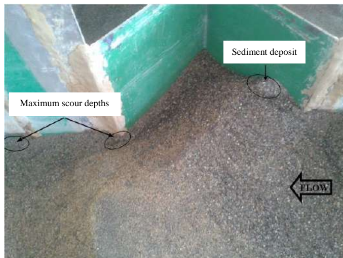
Fig. 4. Sediment deposit and scouring observed in the present study
