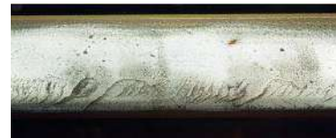
Figure 3. An example of headcheck failure that occur in the rail [16].
