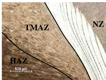
Fig. 4. A cross-sectioned joint comprising three zones (Exp. 6)
