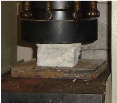
Fig.4 – PAPERCRETE CUBE AFTER COMPRESSION FAILURE
