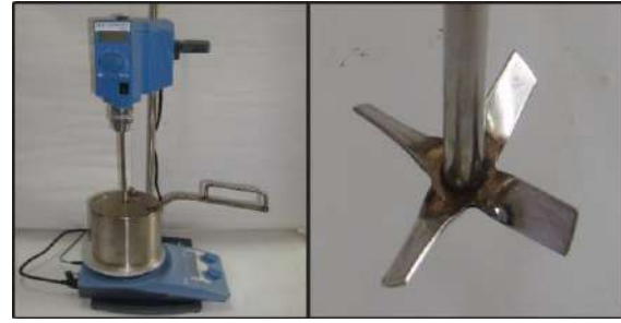
Fig. 1. Modified bitumen mixer and mixing apparatus
