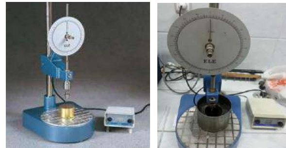
Fig. 2. Penetration test apparatus
