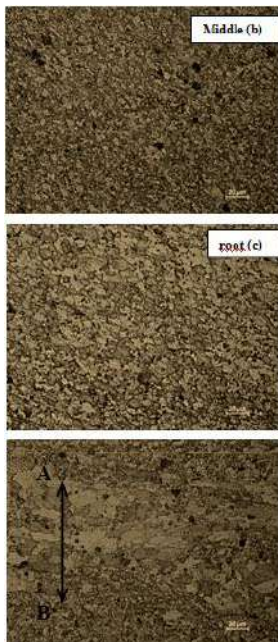
Fig. 6. The changes in the grain size at the nugget zone (threaded pin, 63/630)
