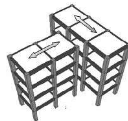
Figure 6. Separating building blocks by seismic joints
