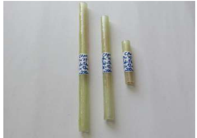
Fig. 1. A test specimens of glass/epoxy
