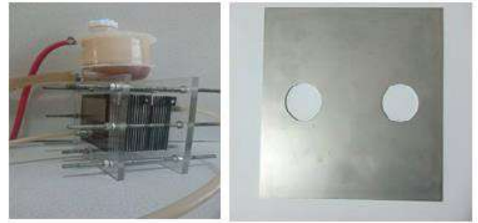
Figure 2. Electrolyzer (left side) and 304L steel plate (right side)
